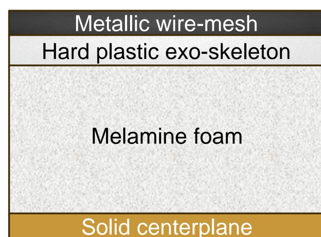
Design and composition of the VKI porous NACA-0024 profile
