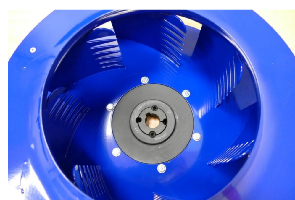
Impeller prototype with LE serrations on the blade
