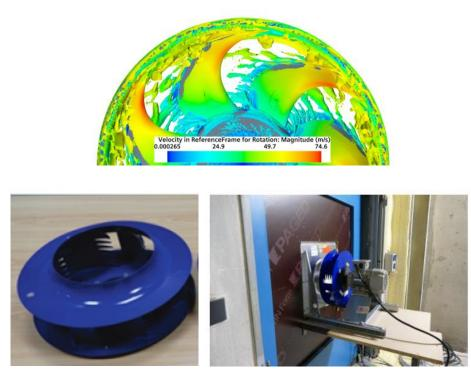
**Excerpt from Deliverable 5.1**: Numerical and experimental research were carried out on the influence of Leading-Edge and Trailing-Edge serrations on aerodynamic and noise performance of a low speed cooling fan industrial application
