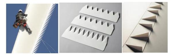
**Excerpt from Deliverable 5.2**: Numerical and experimental research were carried out on the influence of Trailing-Edge serrations and turbulence generators noise performance of wind turbines.
