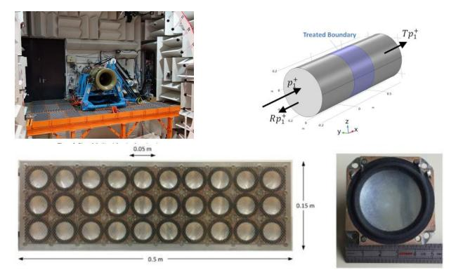
**Excerpt from Deliverable 5.3**: Numerical research was conducted to evaluate the performance of active liners w.r.t state-of-the-art passive liners for reducing ducted sound transmission in a nacelle.
