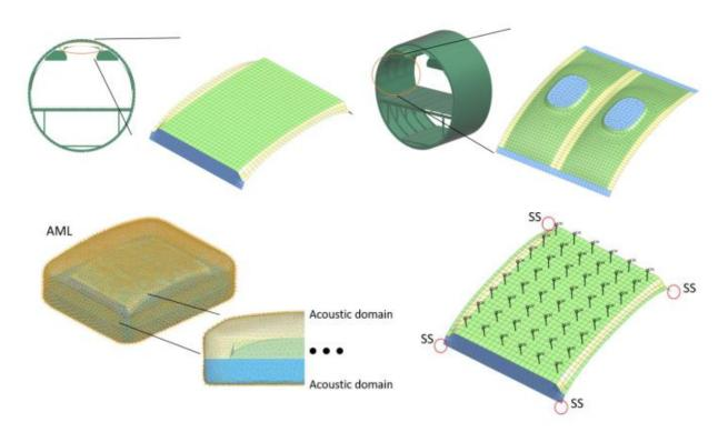
**Excerpt from Deliverable 5.4**: Numerical research was conducted to evaluate the performance of the addition of tuned vibrations absorbers (TVAs) on the fuselage dominant noise transmission paths, in order to improve the noise radiated into the aircraft's cabin
